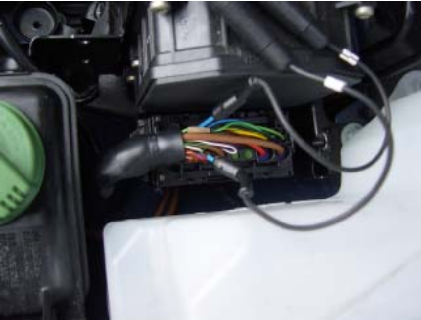
Figure 22 - Connecting the Data Logger to the CAN bus
